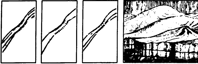
Figure 69. Low Ice Cliff, With Height Less Than Contour Interval. Only those of landmark nature are shown. The tick marks always point downgrade.
